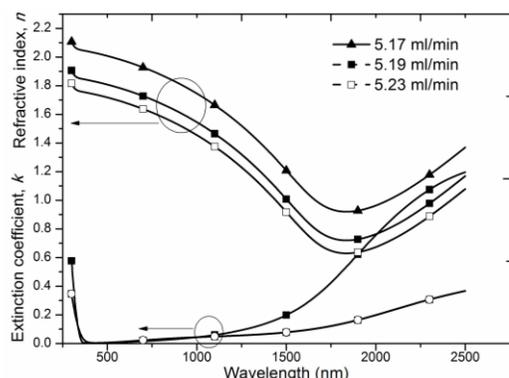
**Figure 3.** Dependence of refractive indices and extinction coefficients of ZnO:Al films on O<sub>2</sub> flow rates.
