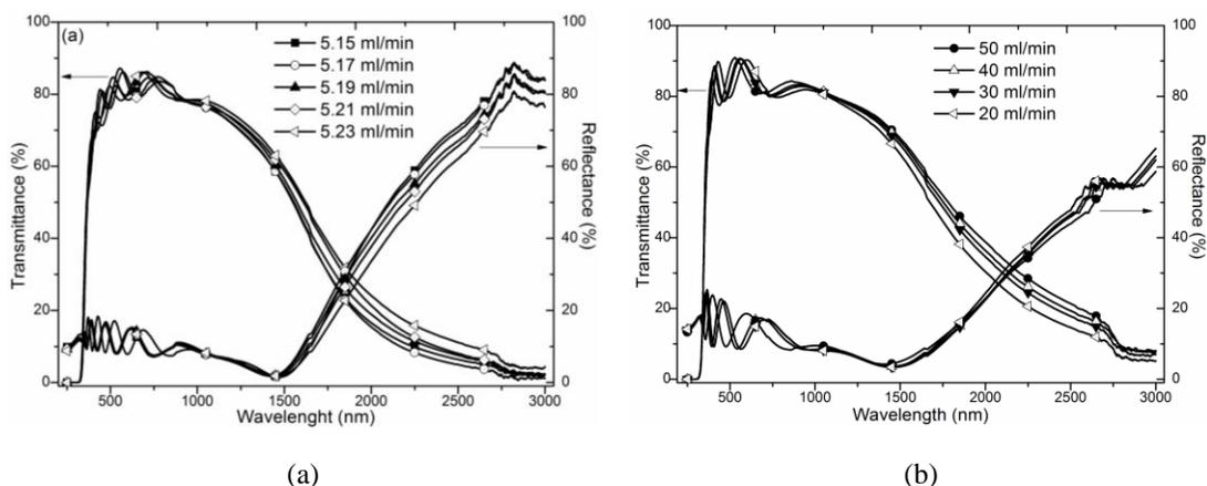
**Figure 2.** (a) Optical transmittance and reflectance spectra of ZnO:Al films grown at various O<sub>2</sub> flow ratio as a mixture of Ar + O<sub>2</sub> gas at 200 °C (b) Optical transmittance and reflectance spectra of ZnO:Al thin films prepared at different argon gas flow rate.
