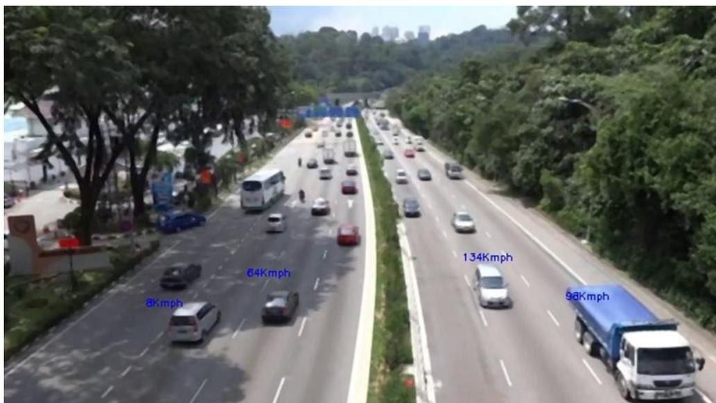
Figure 9: Estimated vehicle speeds using the proposed system.
