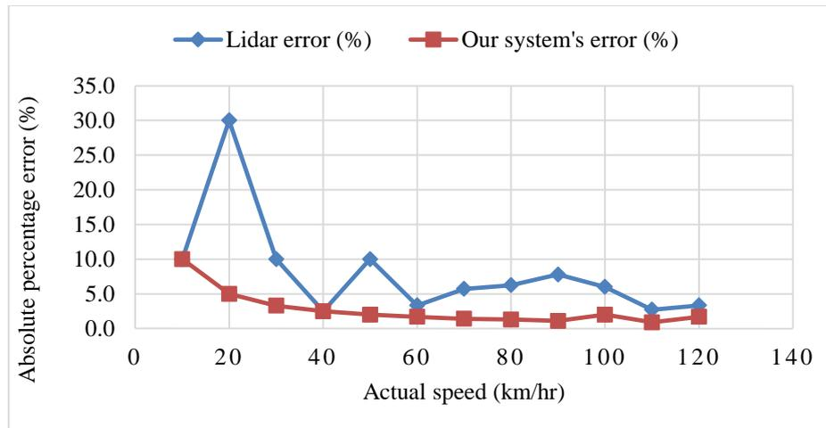
Figure 8: Percentage errors of lidar and proposed systems with frame skipping equals three.
