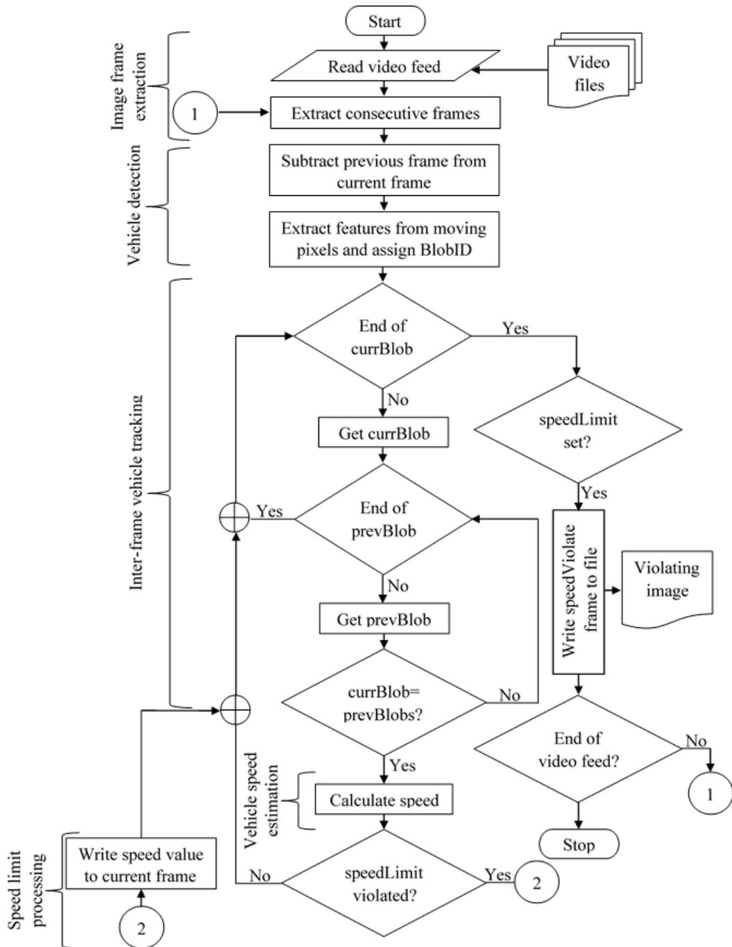
Figure 3: Proposed algorithm for multi-vehicle speed estimation.
