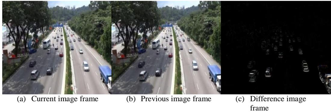
**Figure 5:** Modular system testing of the inter-frame vehicle tracking component.
