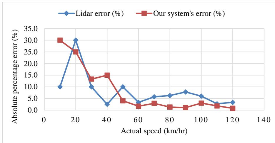
Figure 7: Percentage errors of lidar and proposed systems with frame skipping equals two.
