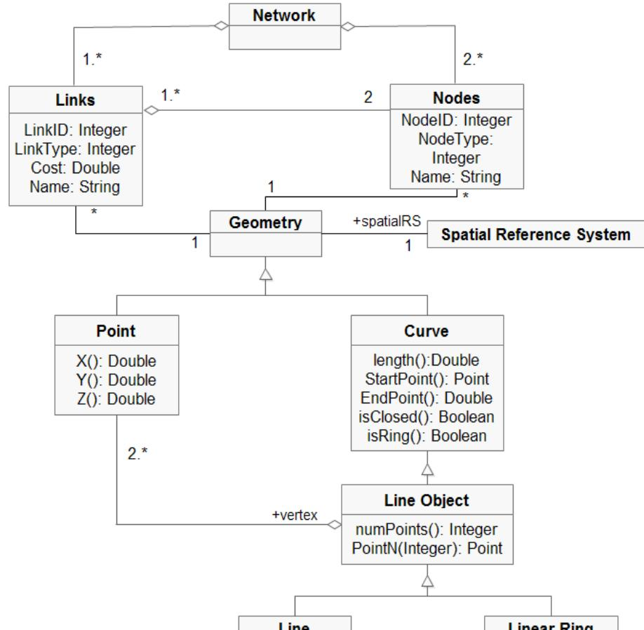
**Figure 3:** UML representation of data structure of route network component.
