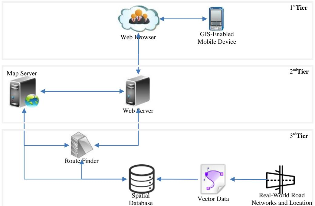
**Figure 2:** Designed pedestrian navigation system (PNS) architectural framework.
