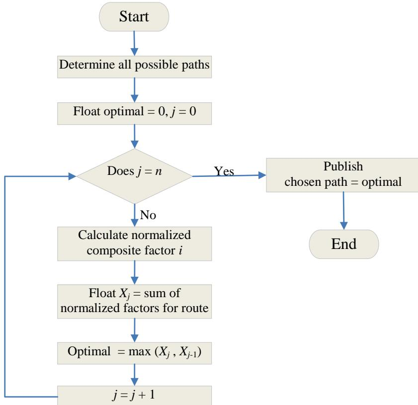
Figure 7: Flowchart for optimal path determination.
