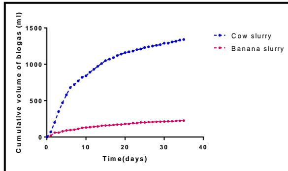
**Figure 3:** Biogas generated from two different inoculums
