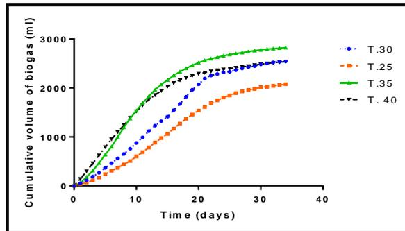
**Figure 5:** Cumulative biogas produced at different temperatures
