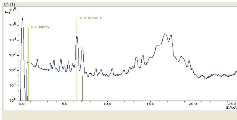
**Figure 3:** Typical Spectrum of Soil Sample Collected in MitooMbuga area
