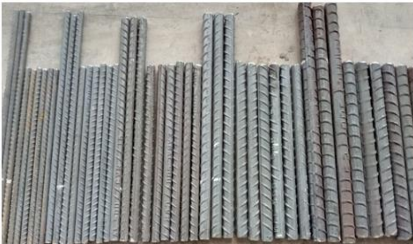
Figure 1: Rebar specimens arranged according to respective nominal diameter size.
