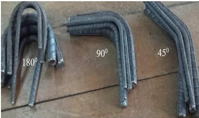
Figure 2: Rebar specimens bent at different angles for different nominal diameter sizes.
