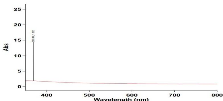
**Figure 2:** Ultra-violet visible spectrum of silver nanoparticles bound.
