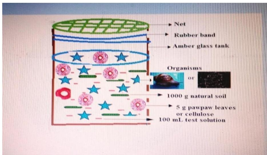
**Figure 1:** Set up for toxicity test.
