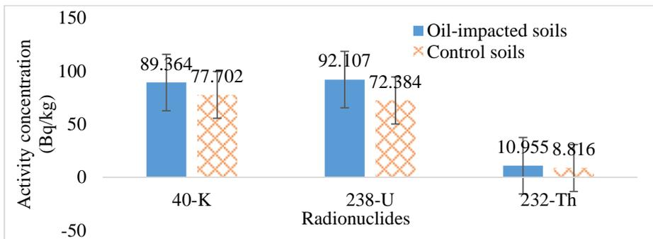
**Figure 2:** Comparison of the activity concentrations of the identified radionuclides in the oil-impacted and control soils.
