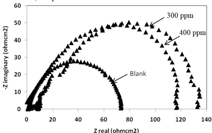
**Figure 2:** Impedance plot in Nyquist format for mild steel electrodes in 0.5 M H<sub>2</sub>SO<sub>4</sub> solutions without and with 300 ppm and 400 ppm concentrations of *Acacia senegal* gum (pH 0.7) at 35 °C.
