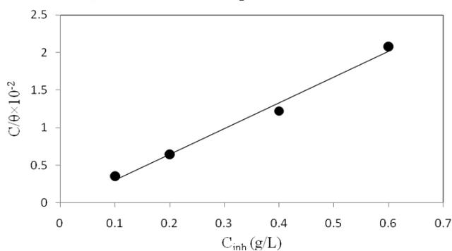
**Figure 6:** Langmuir adsorption isotherm for adsorption of *Acacia senegal* gum on mild steel surface in  $0.5$  M  $H_2SO_4$  solution from impedance data at  $35$  °C.
