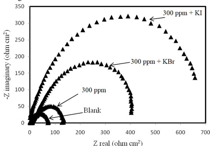
**Figure 4:** Impedance plot in Nyquist format for mild steel electrodes in *Acacia senegal* gum and *Acacia senegal* gum with 0.08 M KBr or 0.08 M KI in 0.5 M  $H_2SO_4$  (pH 0.7) at 35 °C.
