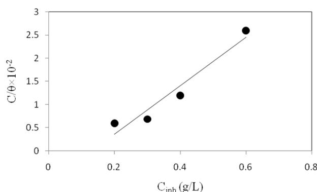
**Figure 5:** Langmuir adsorption isotherm for adsorption of *Acacia senegal* gum on mild steel surface in  $0.5$  M  $H_2SO_4$  solution from polarization data at  $35$  °C.
