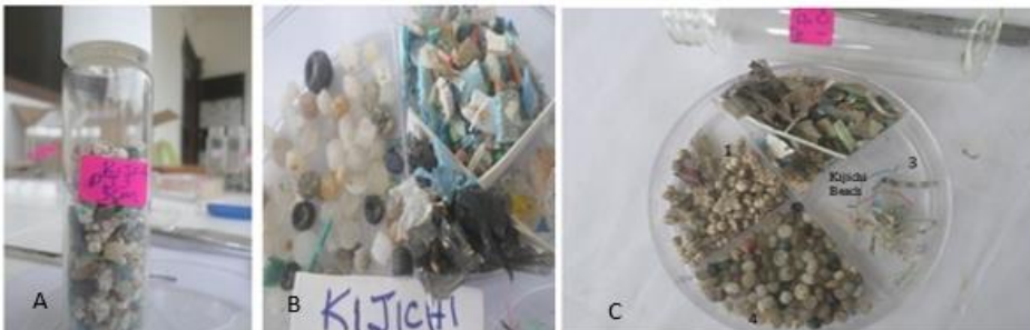
Figure 3: Microplastics in Kijichi Beach. In Figure C, number 1 are sponges, number 2 are fragments, number 3 are fibres number 4 are pellets (nurdles), all found at 1 cm.
